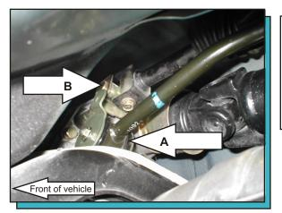
**Note:** Do not remove the upper shifter linkage (See arrow B). Remove old rubber bushing from the lower shifter linkage at the transmission mounting stud. (See arrow A) Install the new poly bushing into the linkage with the part number (1170) facing outward away from transmission.
