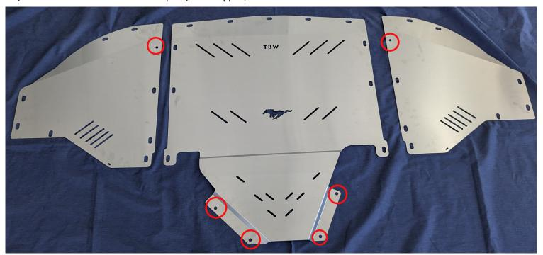
**#5**) Install the side pieces on each side – use three (3) of the M6 bolts to secure each corner piece. U-nuts will be pre-installed on the corner pieces for where the center section overlaps
