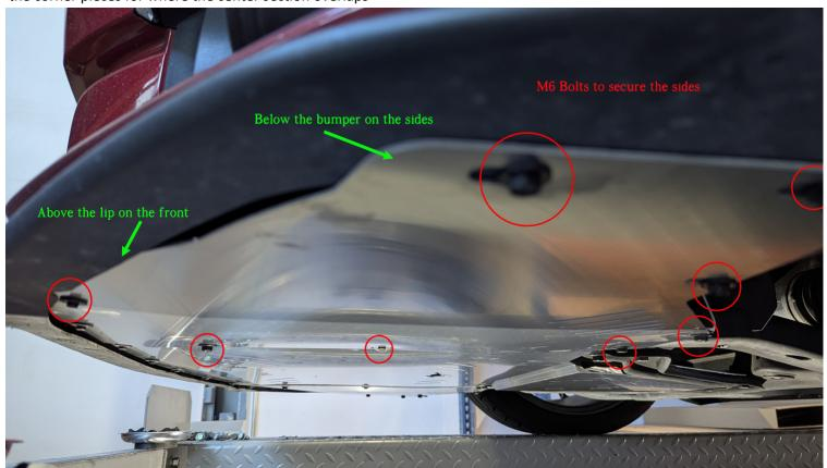
**#6)** Install the middle (main) panel. Secure the aluminum with M6 bolts - five (5) will be used along the front bumper, four (4) through the V-brace that attach to u-nuts installed in step #4
