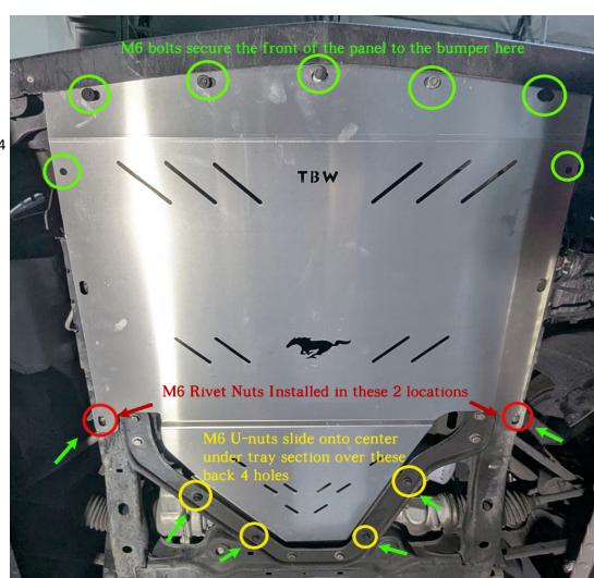
**#7)** At this point all bolts should be in place. With bolts all in position you can tighten them down to 15-20 ft lbs (snug).
