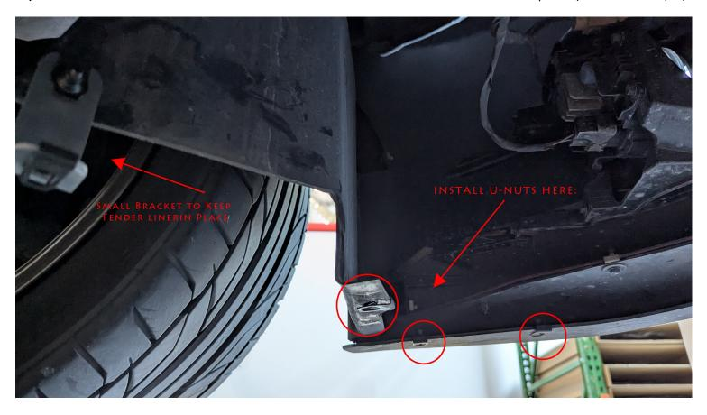
**#3**) Install the two(2) M6 Rivet nuts in the existing holes in the chassis
