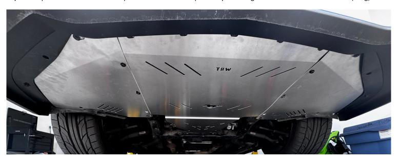
WITH ALL BOLTS IN PLACE – TIGHTEN DOWN TO APPROX 15-20 FT LBS. Do NOT tighten any bolts down until ALL are in place
