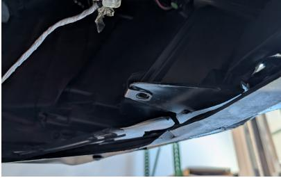
**#4**) Install the Corner pieces on each side – use three (3) of the M6 bolts to secure each corner piece. U-nuts will be preinstalled on the corner pieces for where the center section overlaps
