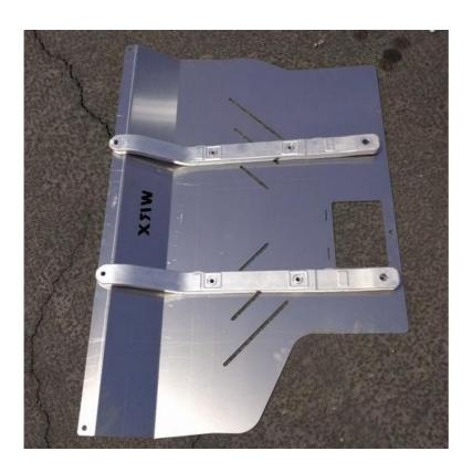
**#3)** Install the 6mm Extruded U-nuts in the marked location here. The other 4 will be used on the front bumper holes to make a much stronger install than the plastic push clips.
