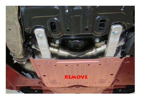
**#2)** You will want to align the metal brackets with the holes on the under tray. This can be easier with them off of the car but is not necessary. You will utilize the oem bolts and lock nuts here. Just put them on hand tight so you have a little flexibility for aligning the rest of the bolts to their holes.
