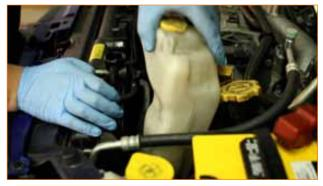
6. Disconnect the electrical harnesses for the fans.
