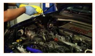
$\pmb{6}.$  Start the vehicle, set the heat to high, and check for leaks and power to the fan.
